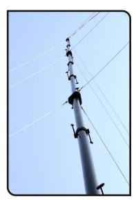
The pneumatic telescopic mast is a structure used to raise the payload to an operational level. It consists of several concentric, nesting mast sections, fabricated from special grade, light weight made of high tensile alloy aluminum extruded tubes that extend and retract pneumatically. Pneumatic masts are ideal for military communications, surveillance, elevated testing, mobile radar, areal photography and meteorological applications etc.
